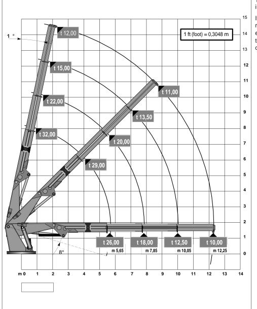
The diagram refers to the using of the crane. in sea state '0, or in a harbour condition.
