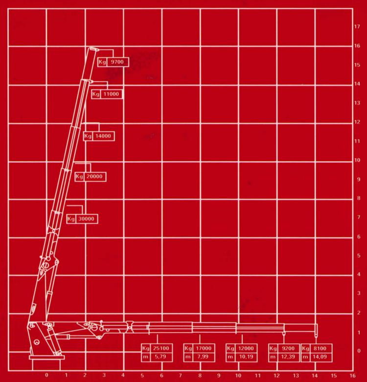
DIAGRAM REFERRED TO CRANE AT "0" SEA ROUGHNESS OR AT HARBOUR CONDITION IF THE CRANE IS USED OFF SHORE IN ROUGHER SEA CONDITIONS, CONTACT THE SUPPLIER TO ESTABLISH LOADING CAPACITIES OR REDUCTION PARAMETERS.
